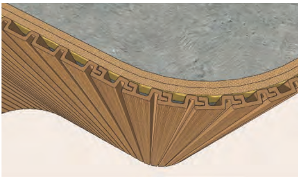
Vertical installation on convex curved wall with a minimum radius of 1m
