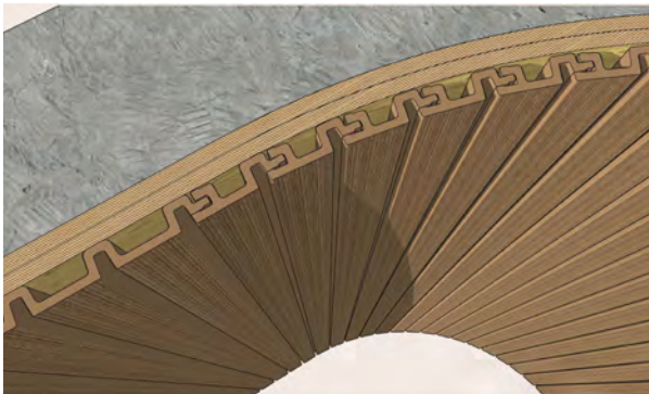
Vertical installation on concave curved wall with a minimum radius of 1m
