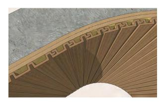
Vertical installation on concave curved wall with a minimum radius of 1m
